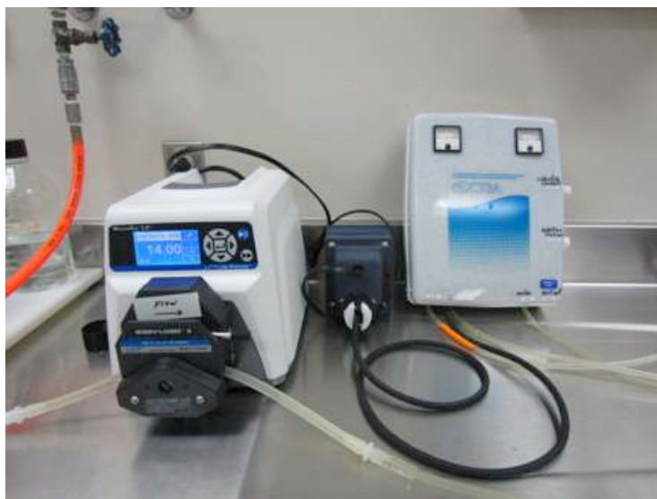
Figure 4.6. Photograph of STEL Device Connected to the Peristaltic Pump
